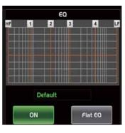
Touch the switch ON to enable EQ function, it will illuminate and synchronize with ON/OFF control in EQ page. Please set values in EQ page because it is not adjustable here. This page can only show the values. You can also load a preset, please refer to load introduction section for the detail operation, the loaded state will show in the middle box.
