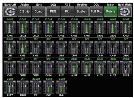
This icon indicates current channel's fader position, "0" is zero dB position.
