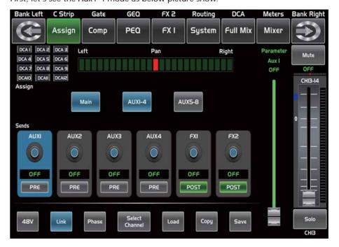
Touch Main, AUX1-4 or AUX5-8 on the LCD screen or corresponding button on the panel to assign input channel audio to these channels or buses. They
