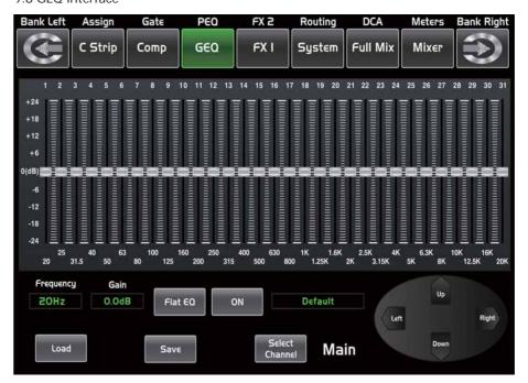
The digital mixer features MAIN Stereo, AUX Mono, 31-band, 1/3 octave graphic EQs. The 31 bands range from 20Hz to 20 KHz. There is 1 MAIN Stereo GEQ, 8 AUX Mono GEQs in 24-bit/48 kHz sample rate.
