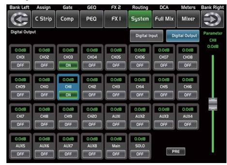
When you select a channel as digital output, OFF will switch to ON, the background of ON will illuminate. The screen will give clues if no digital card inserted in, and the Digital Out function can not enable either.
